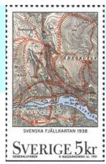
Contours are drawn at equal intervals, say every 100ft. A series of concave lines indicates a valley, convex lines an outcrop. Wide spacing shows flat ground and close spacing a slope.
